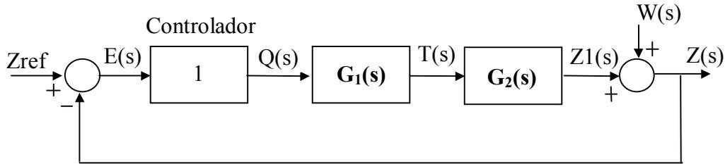
$$G_1(s) = \frac{T(s)}{Q(s)} = \frac{1}{s+5} \quad G_2(s) = \frac{Z_1(s)}{T(s)} = \frac{0.3}{s(s+50)}$$
