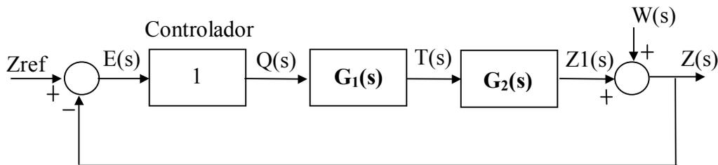
$$G_1(s) = \frac{T(s)}{Q(s)} = \frac{1}{s+5} \quad G_2(s) = \frac{Z_1(s)}{T(s)} = \frac{0.3}{s(s+50)}$$
