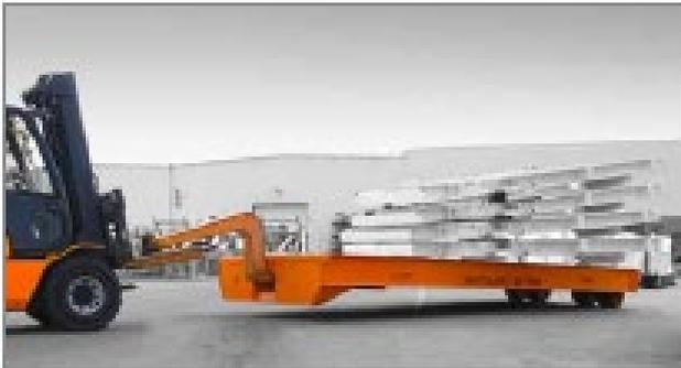
» Cargo trailer system with forklift truck
