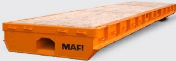
Rolltrailers are used by terminal operators all over the world. They are mostly in operation to load/unload general cargo and standard ISO containers on/off the various ships. As equipment with different shapes and sizes arrive at the port the rolltrailers can be manufactured accordingly. Rolltrailers will be your perfect "tool" for handling overheight cargoes, very heavy loads or odd pieces.
