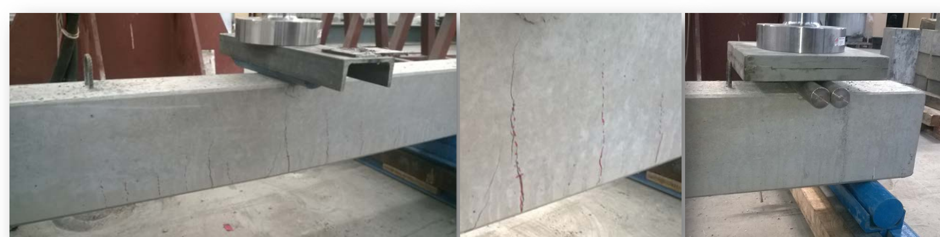
Three points and shear testing on a reinforced recycled beam performed on the laboratory.
