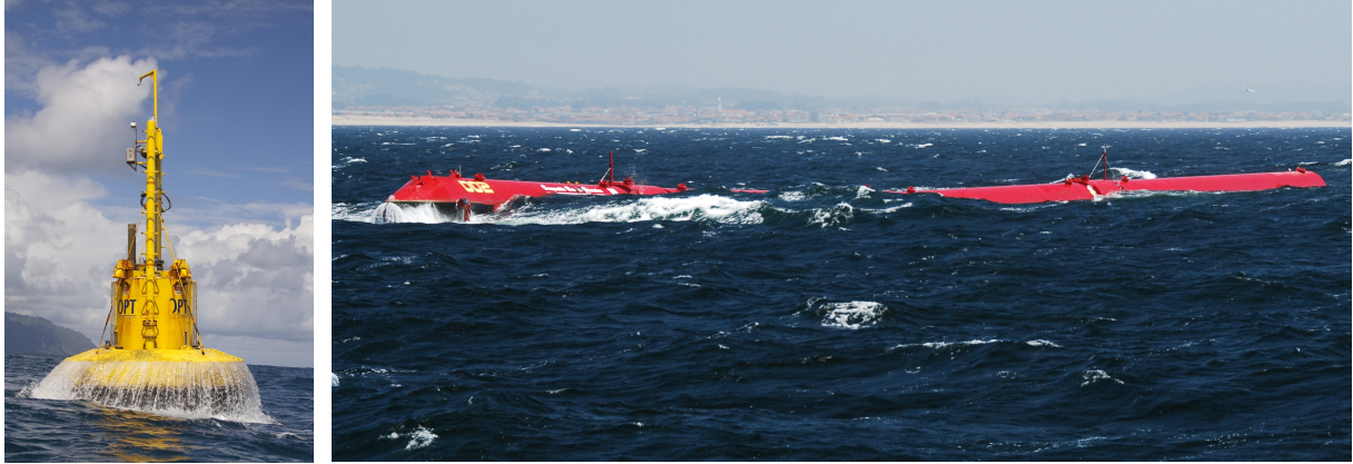
Figure 3. Devices for utilizing wave power (left: PB40 PowerBuoy by Ocean Power Technologies (License: Public Domain); right: Pelamis machine (License: Public Domain)).
