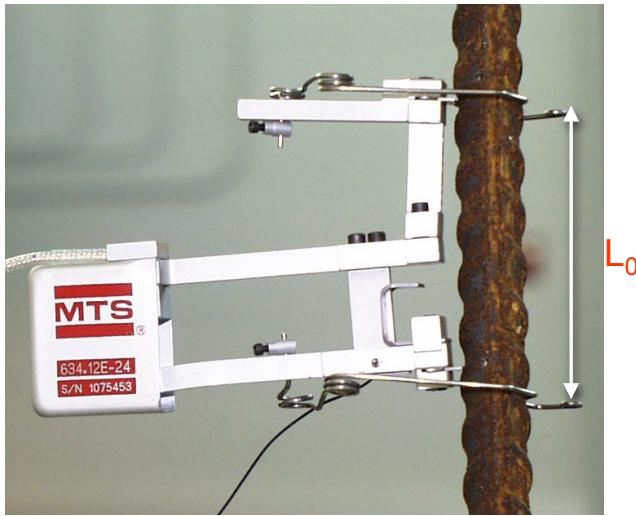
Pin extensometer (with contact).
