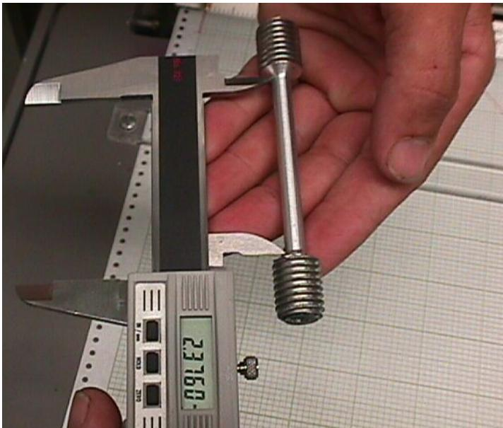
Determine the **initial cross section ( $A_0$ )** of the specimen to calculate the **reduction in area** after the test.
