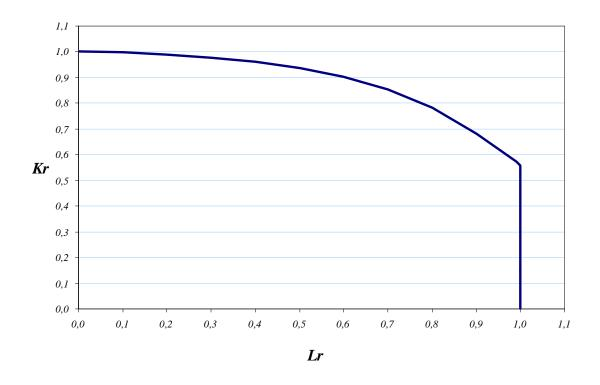
**4.** The quality department of a company that manufactures automobiles, aims to study the behavior of a large metal plate that is a part of the frame of a motor. In this kind of components, there has been systematically reported the existence of fatigue problems from edge cracks. As this is a very carefully fabricated element that has passed very strict inspections, the presence of initial cracks can be dismissed.
