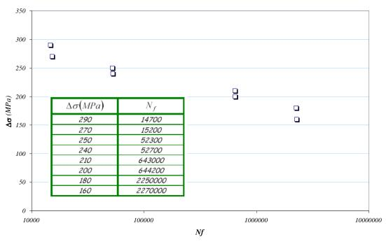
Once the material has been characterized, it is decided to study the problematic behavior in operating conditions. It is known that, on average, the component is subjected every day to three sequences of 10000 cycles each one, with  $\Delta \sigma = 100$ , 125 and 150 MPa, respectively, being  $\sigma_m = 50 MPa$ . These sequence repeats indefinitely.
