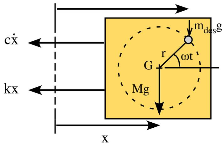
$$-c\dot{x} - kx = M\ddot{x} + m_{des} \frac{d^2(x + r \cos \omega t)}{dt^2}$$
