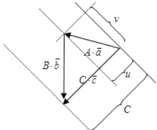
$$\left. \begin{aligned} A^2 &= u^2 + v^2 \\ B^2 &= (C - u)^2 + v^2 \end{aligned} \right\} \quad u = \frac{A^2 + C^2 - B^2}{2 \cdot C} \quad v = \pm \sqrt{A^2 - \left(\frac{A^2 + C^2 - B^2}{2 \cdot C}\right)^2}$$
