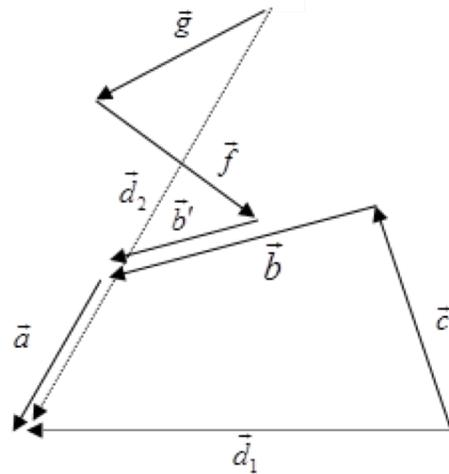
$$\left. \begin{aligned} \vec{g} + \vec{f} + \vec{b}' + \vec{a} &= \vec{d}_2 \\ \vec{c} + \vec{b} + \vec{a} &= \vec{d}_1 \end{aligned} \right\}$$
