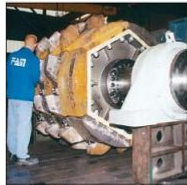
Crushing roll heavy-duty type diameter 2000 mm
