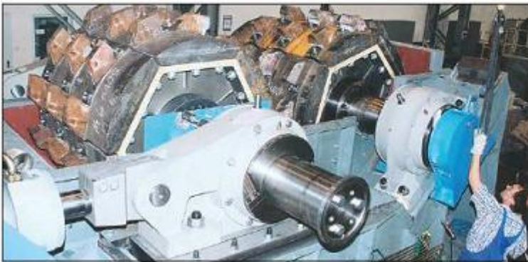
Double roller crusher SZWB2015 heavy-duty type rotor diameter 2000 mm rotor width 1500 mm input 0 - 900 mm output 0 - 200 mm
