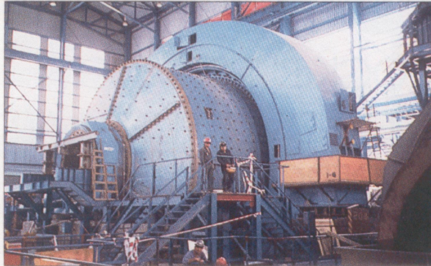
The world's largest operating SAG mill is a 36-ft-dia. × 15-ft unit, driven by a 15,000-hp wrap-around motor.
