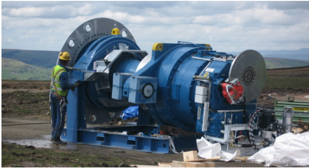
Figure 47. Detail of brake (and gear box and rotor shaft) assembly for a Nordex N80 wind turbine (tower height: 60 m; blade length: 40 m). Source: Paul Anderson (CC BY-SA 2.0). http://bit.ly/2ES1HbK
