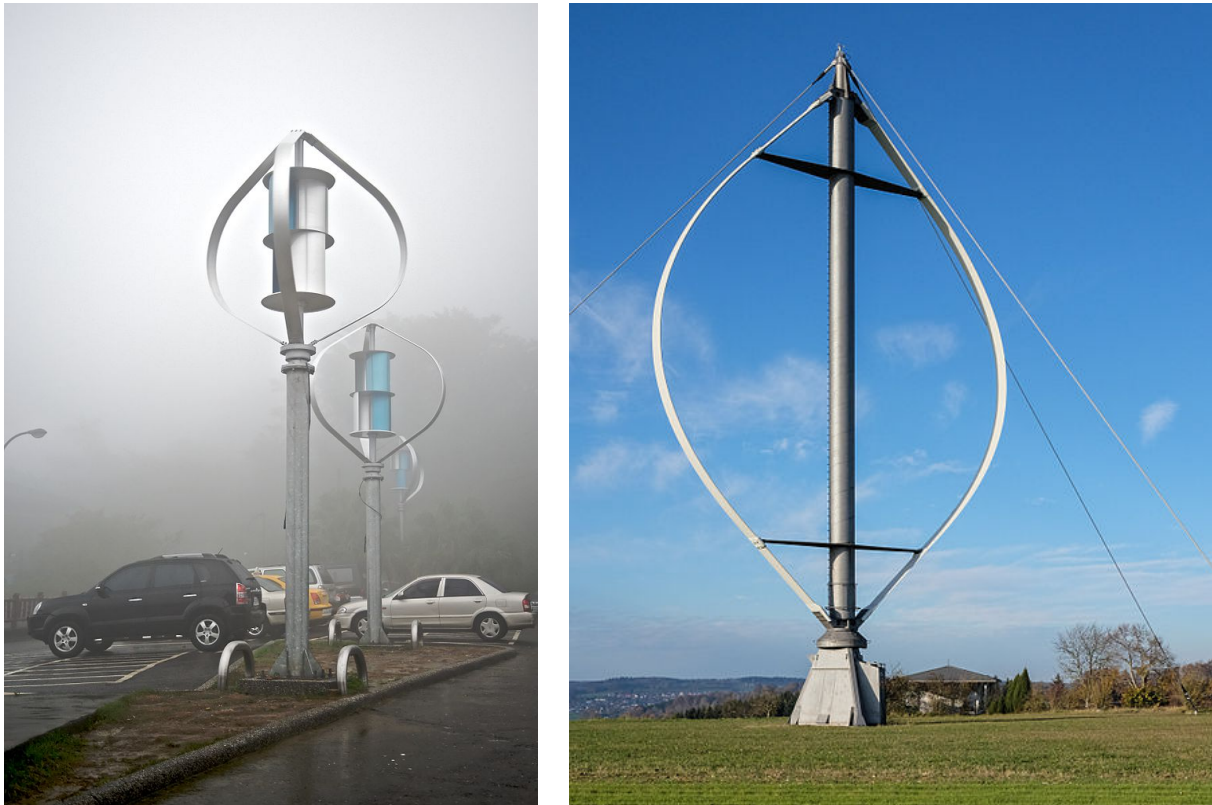
Figure 3. Savonius and Darrieus wind turbines: Savonius wind turbine in Taiwan (left); Darrieus wind turbine in Baden-Württemberg (Germany). Source (left): http://bit.ly/2mG2mWV (License: CC BY-SA 3.0 (Attribution: Dietrich Krieger)); Source (right): http://bit.ly/2mAbNXf (License: CC BY-SA 3.0).
