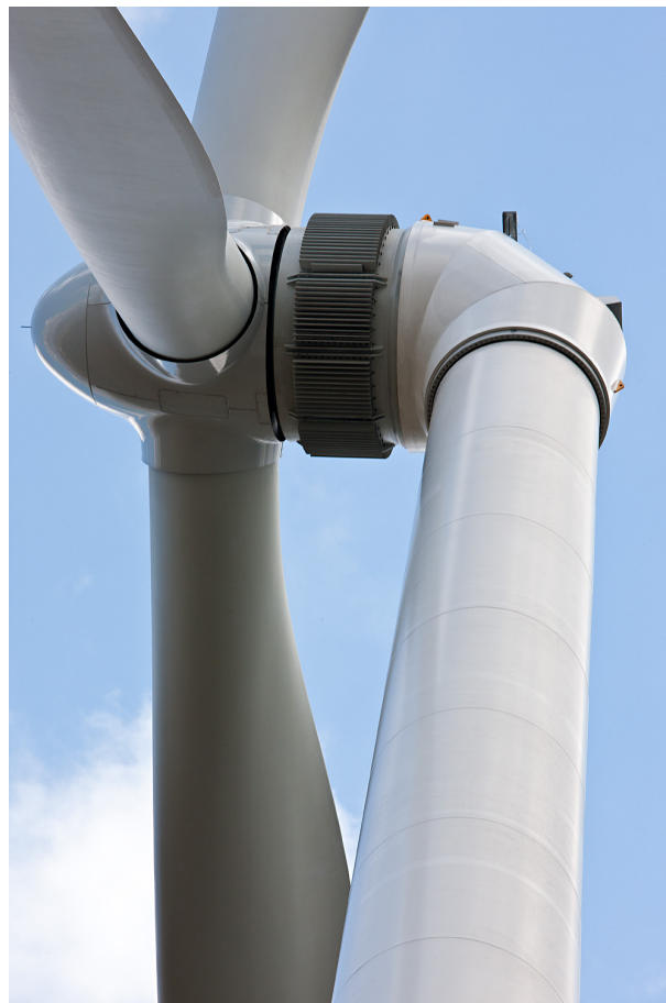
Figure 57. Direct-drive wind turbine. Source: Wikimedia. License: CC BY-SA 2.5 http://bit.ly/2Dex1Rn
