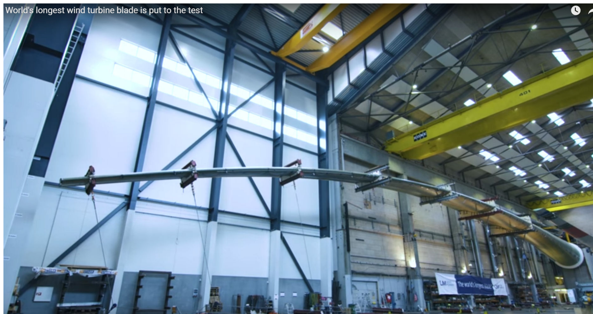
Figure 1.58. Image of the blade test of a wind turbine blade measuring 88.4 meters long. Source: LM Wind Power. Frame of the YouTube video: https://youtu.be/5m-jwwM3qRs
