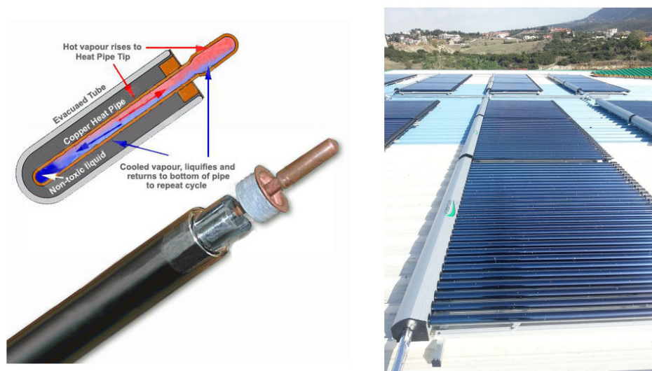
Figure 2.7. Working principle of evacuated tube collectors (left). Example of solar thermal system based on evacuated tube (right). Source (left): http://bit.ly/2kUyt3x (Public Domain). Source (right): Green-solarvacuum (License: CC-BY-SA 3.0) http://bit.ly/2kW0Gqv .
