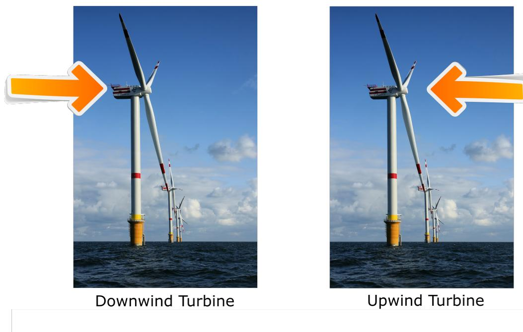
Figure 3.39. Upwind and downwind turbines. Source: Wikimedia. License: CC BY-SA 4.0 Attribution © Hans Hillewaert) <http://bit.ly/2EPJ0Fp>.
