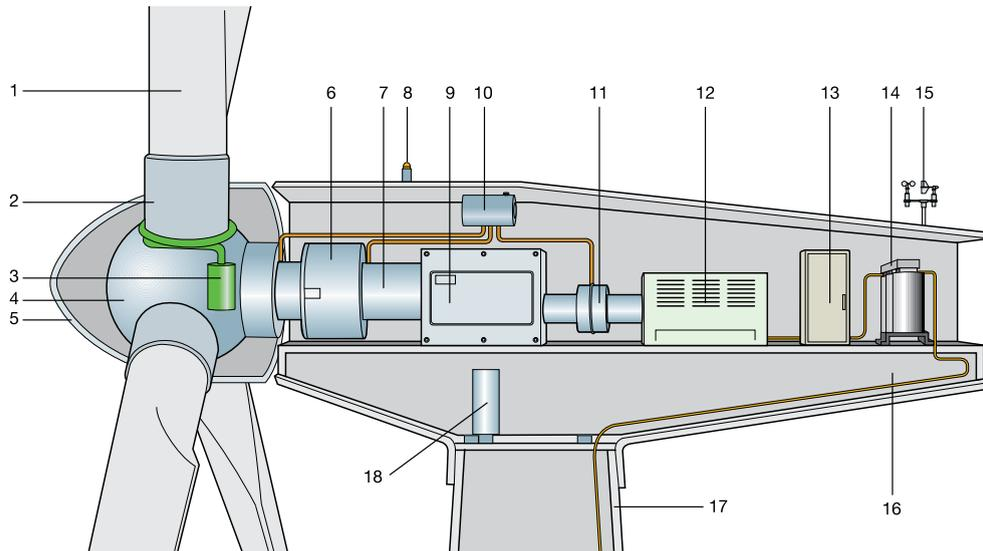
**Figure 3.27.** Components of a wind turbine. Source: Plantas eólicas/ABB Cuaderno técnico.
