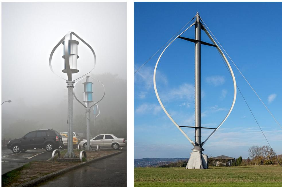
**Figure 3.3.** Savonius and Darrieus wind turbines: Savonius wind turbine in Taiwan (left); Darrieus wind turbine in Baden-Württemberg (Germany). Source (left): <http://bit.ly/2mG2mWV> (License: CC BY-SA 3.0 (Attribution: Dietrich Krieger)); Source (right): <http://bit.ly/2mAbNXf> (License: CC BY-SA 3.0).
