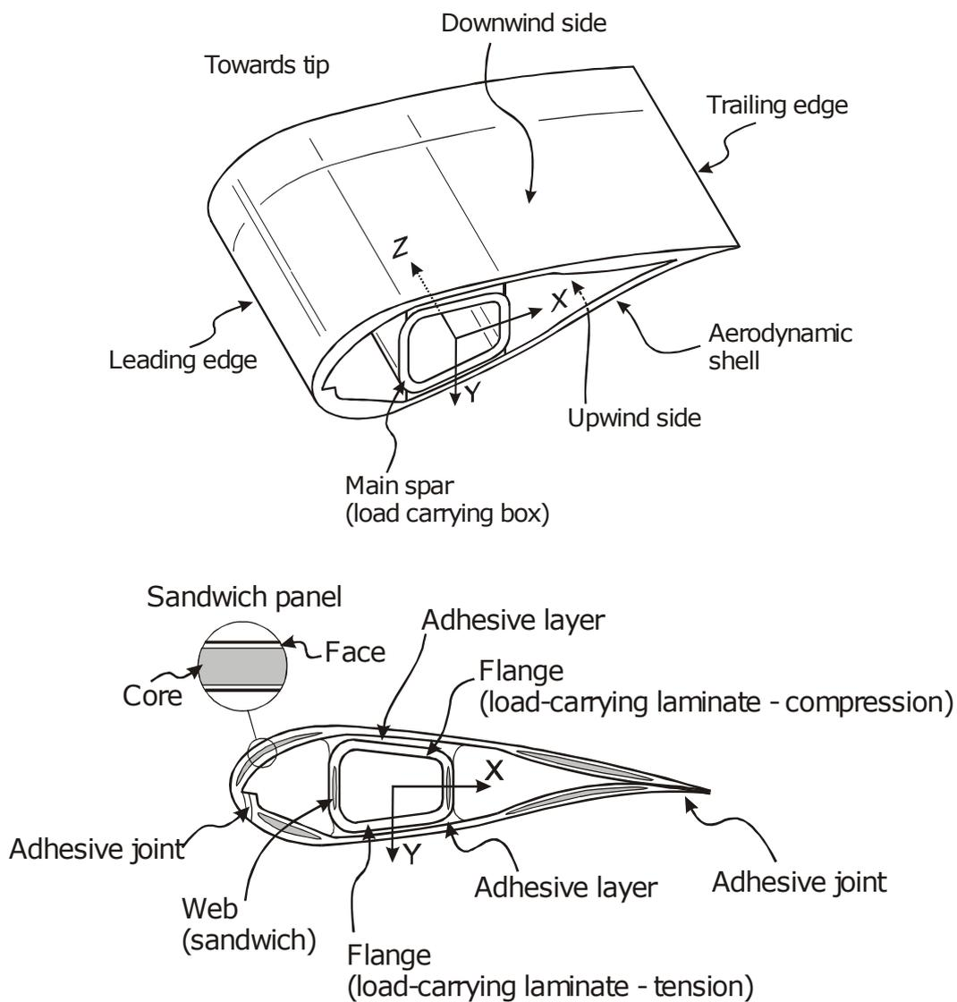
**Figure 3.33.** Detail of the cross-section of a wind turbine blade. Source: Riso R-1390: *Improved design of large wind turbine blade of fibre composites based on studies of scale effects (Phase 1) - Summary Report.*
