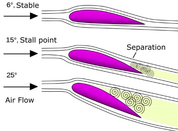
**Figure 3.23.** . Wing stall in terms of angle of attack. Source: Wikimedia <http://bit.ly/2mCu8mg> (Public Domain).
