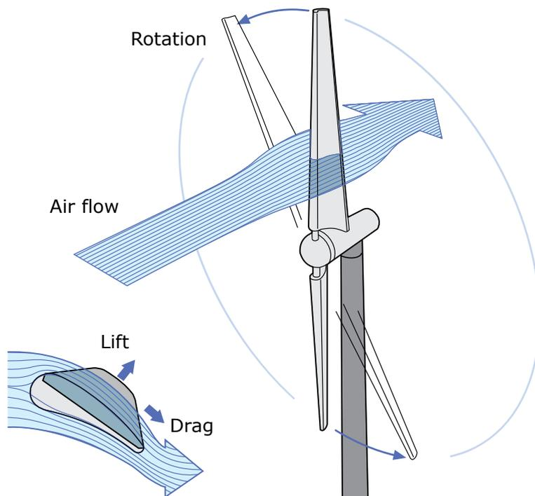
**Figure 3.20.** Working principle of a wind turbine: lift and drag forces. Source: Plantas eólicas/ABB Cuaderno técnico.
