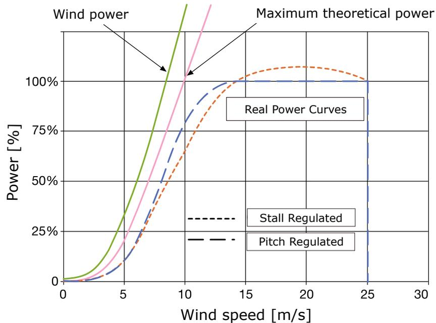
**Figure 3.25.** Wind speed versus output power in a wind turbine. Source: Plantas eólicas/ABB Cuaderno técnico.
