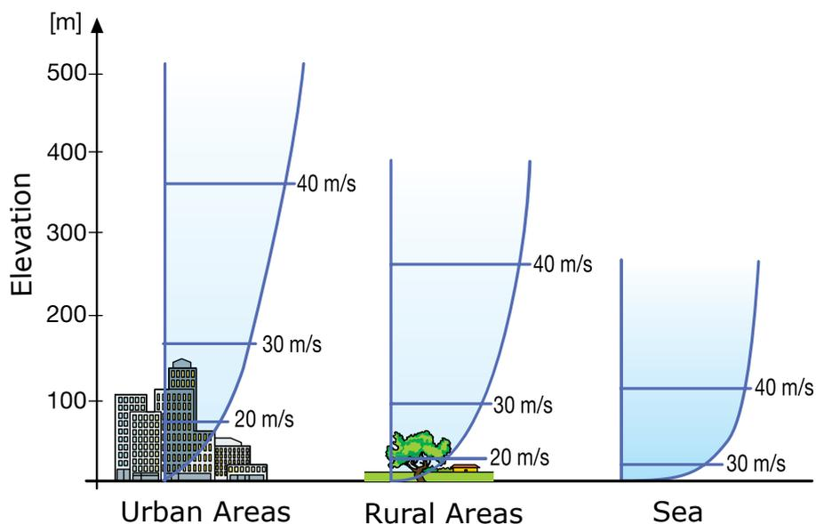
Figure 3.13. Effect of surface roughness on wind speed. Source: Plantas eólicas/ABB Cuaderno técnico.
