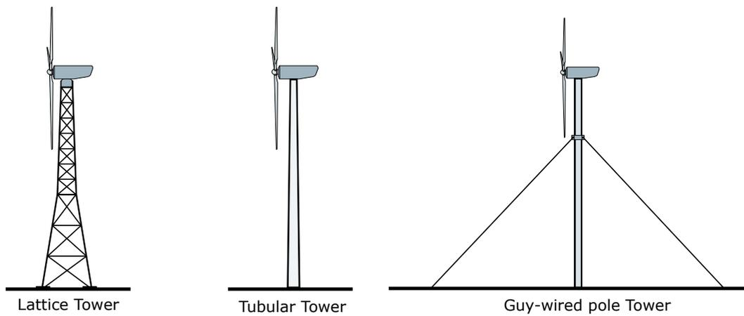
**Figure 3.29.** Tower designs for wind turbines. Source: Plantas eólicas/ABB Cuaderno técnico.
