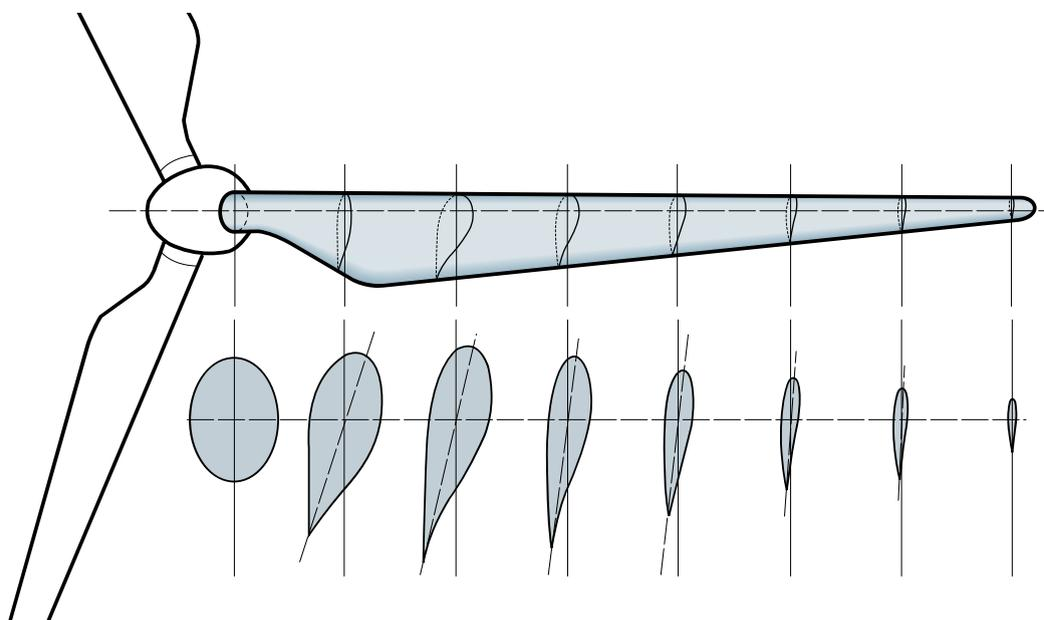
**Figure 3.32.** Blade profile from base to tip: cross-section. Source: Plantas eólicas/ABB Cuaderno técnico.
