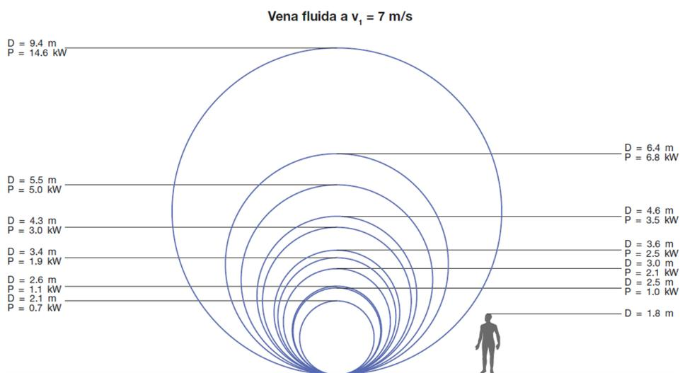
Figure 3.15. Wind turbine generated power in terms of wind speed and rotor diameter. Source: Plantas eólicas/ABB Cuaderno técnico.
