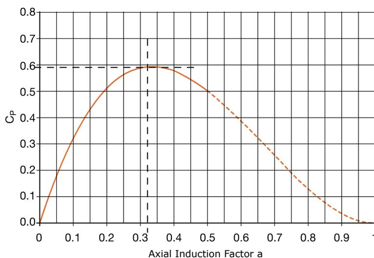
**Figure 3.18.** Power coefficient  $C_p$  versus the axial induction factor  $a$ . Source: Plantas eólicas/ABB Cuaderno técnico.
