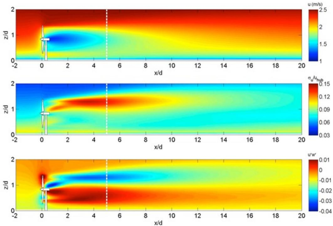
**Figure 3.14.** Turbulence at the back side of a wind turbine. Source: Wind Engineering and Renewable Energy Laboratory Wire <http://bit.ly/2EMfh0n>
