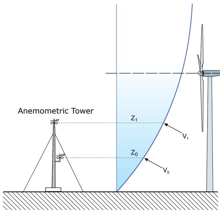
Figure 3.12. Wind speed increase with height. Source: Plantas eólicas/ABB Cuaderno técnico.
