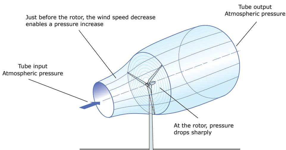
Figure 3.16. Schematic representation of the air mass going through a wind turbine. Source: Plantas eólicas/ABB Cuaderno técnico.
