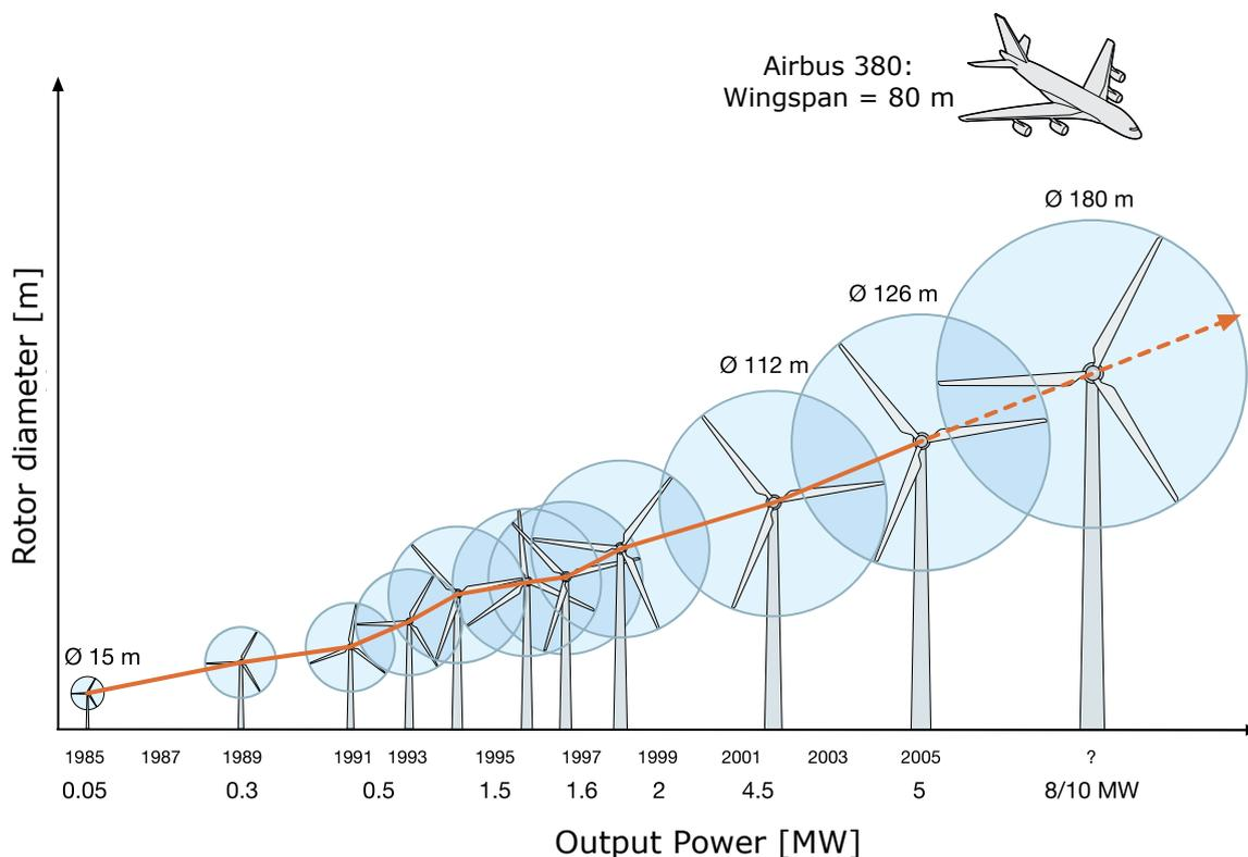
**Figure 3.24.** Rotor size versus output electrical power: evolution over the previous years. Source: Plantas eólicas/ABB Cuaderno técnico.
