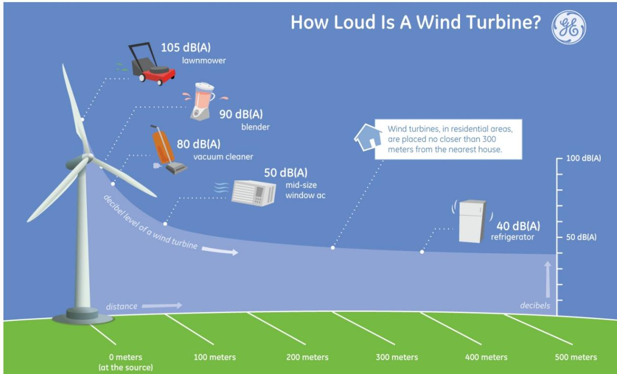
**Figure 3.5.** Noise generated by a wind turbine. Source: GE Global Research / National Institute of Deafness and Other Communication Disorders.
