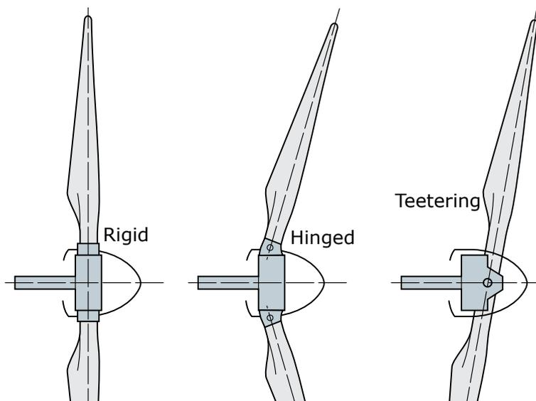
**Figure 3.37.** Hub types for wind turbines: rigid, hinged and teetering. Source: Plantas eólicas/ABB Cuaderno técnico.
