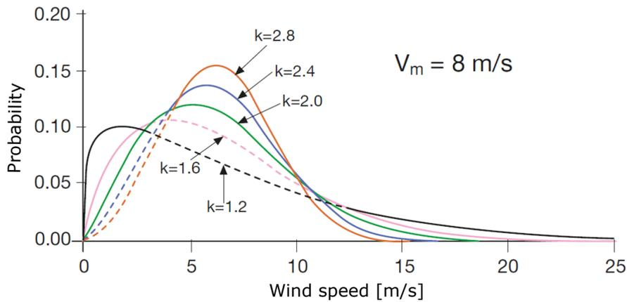
**Figure 3.11.** Weibull distributions for an average wind speed of 8m/s and different values of  $k$ .
