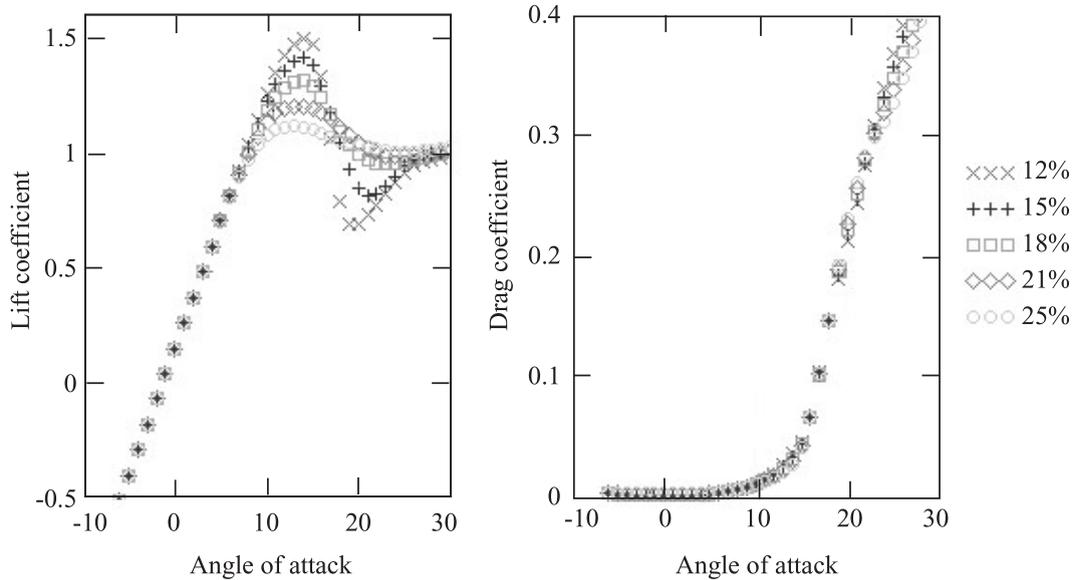
**Figure 3.22.** Evolution of lift and drag coefficients in terms of the angle of attack. Source: Wind Energy Handbook (Wiley), p. 94.
