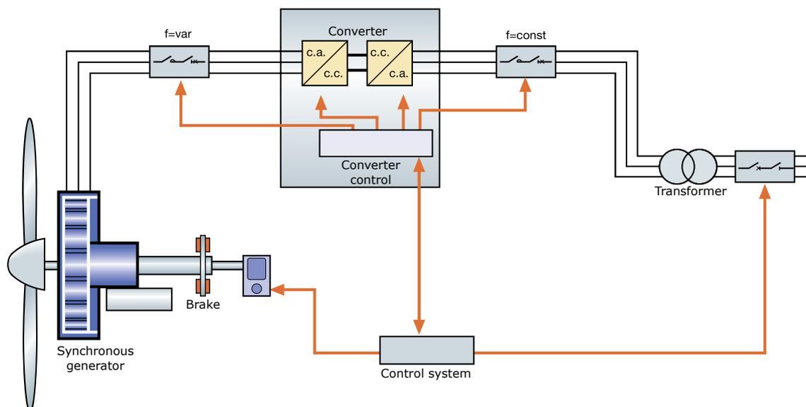
**Figure 3.43.** Schematic representation of a variable-speed wind turbine with synchronous generator. Source: Plantas eólicas/ABB Cuaderno técnico.
