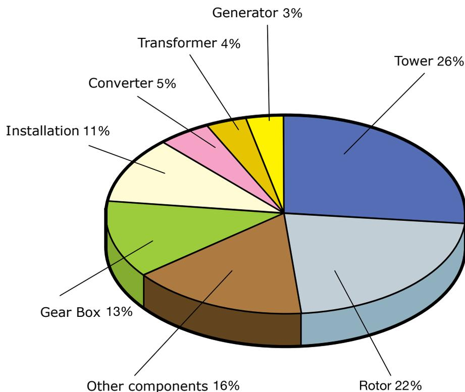
**Figure 3.28.** Cost associated with wind turbine components. Source: Plantas eólicas/ABB Cuaderno técnico.
