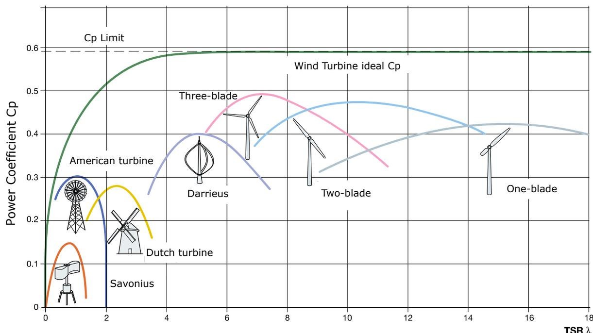
**Figure 3.26.** Power coefficient versus tip speed ratio for different wind turbine models. Source: Plantas eólicas/ABB Cuaderno técnico.
