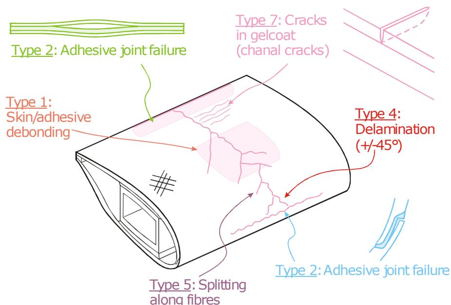
**Figure 3.34.** Detail of the cross-section of a wind turbine blade: possible defects. Source: Riso R-1390: *Improved design of large wind turbine blade of fibre composites based on studies of scale effects (Phase 1) - Summary Report.*
