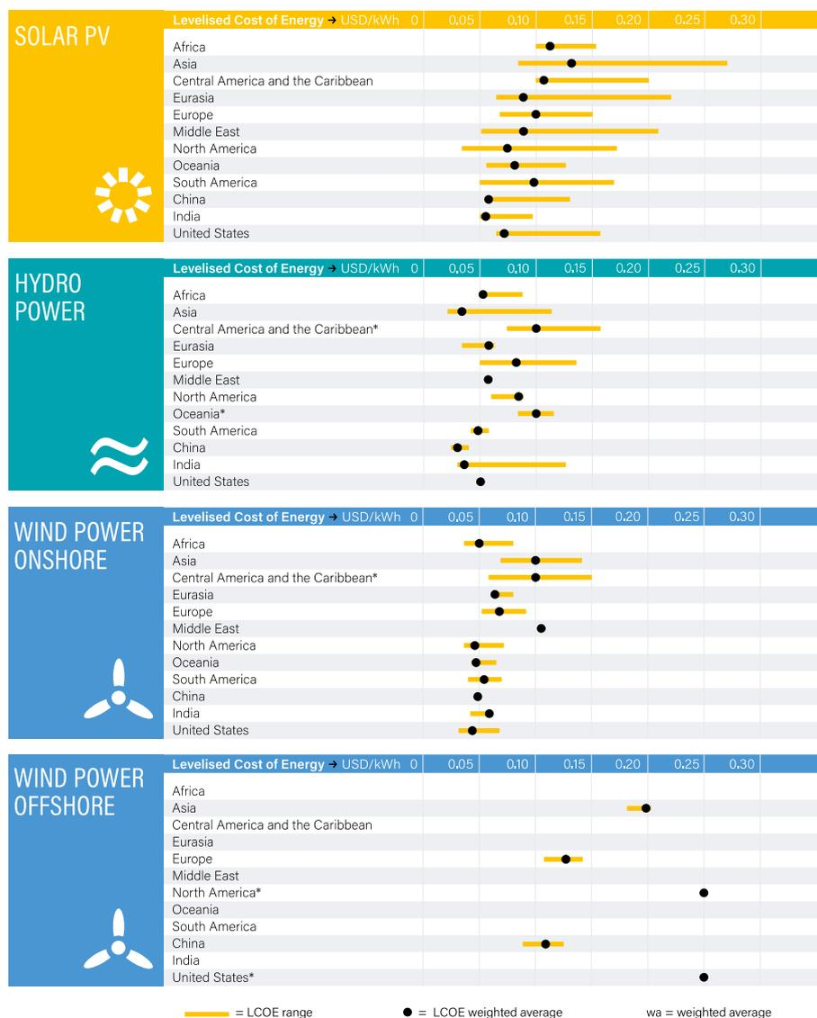
**Figure 3.7.** LCOE for hydro and wind power (2018). Source: Renewables 2019 Global Status Report (REN21). <http://bit.ly/2rTdy3>
