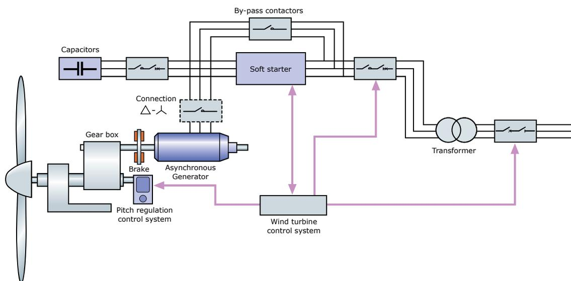
**Figure 3.42.** Schematic representation of a fixed-speed wind turbine. Source: Plantas eólicas/ABB Cuaderno técnico.
