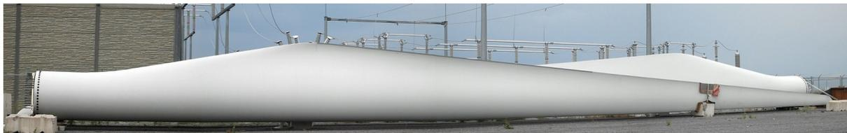
**Figure 3.31.** Siemens wind turbine blade (49 m long). Source: Wikimedia. License: CC BY-SA 3.0. <http://bit.ly/2DrA646>
