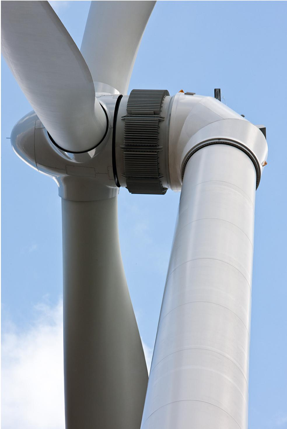
**Figure 3.45.** Direct-drive wind turbine. Source: Wikimedia. License: CC BY-SA 2.5 <http://bit.ly/2Dex1Rn>
