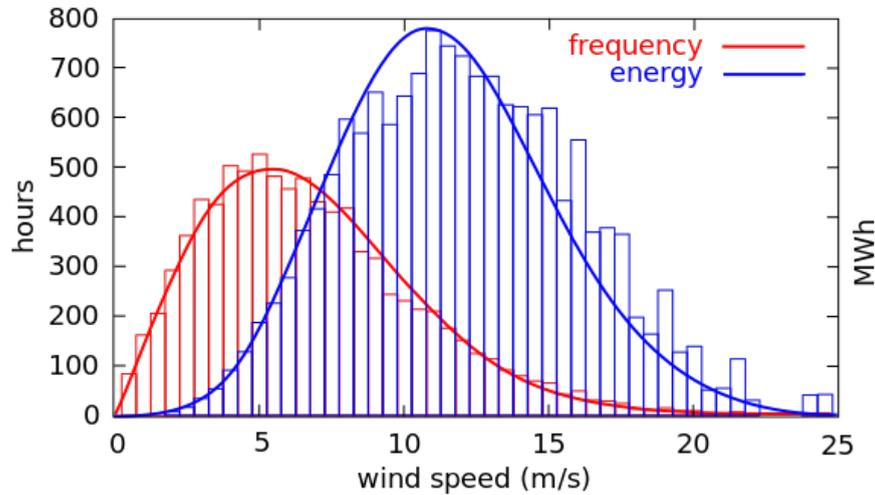
**Figure 3.10.** Example of Weibull distribution (red) used to model wind speed data. The energy produced by the wind turbine has been represented in blue. Source: <http://bit.ly/2FEQZGz>. License: CC-BY-SA 3.0.
