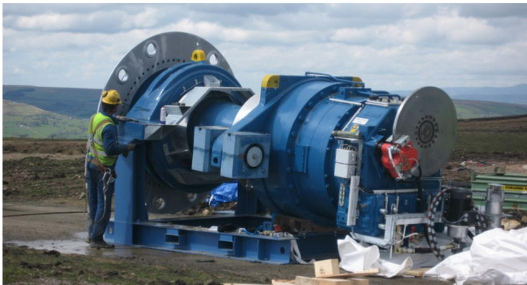
**Figure 3.41.** Detail of brake (and gear box and rotor shaft) assembly for a Nordex N80 wind turbine (tower height: 60 m; blade length: 40 m). Source: Paul Anderson (CC BY-SA 2.0). <http://bit.ly/2ES1HbK>
