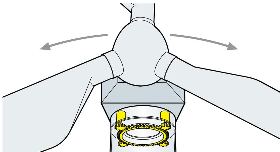
Figure 3.38. Yaw system in a horizontal-axis wind turbine. Source: Plantas eólicas/ABB Cuaderno técnico.
