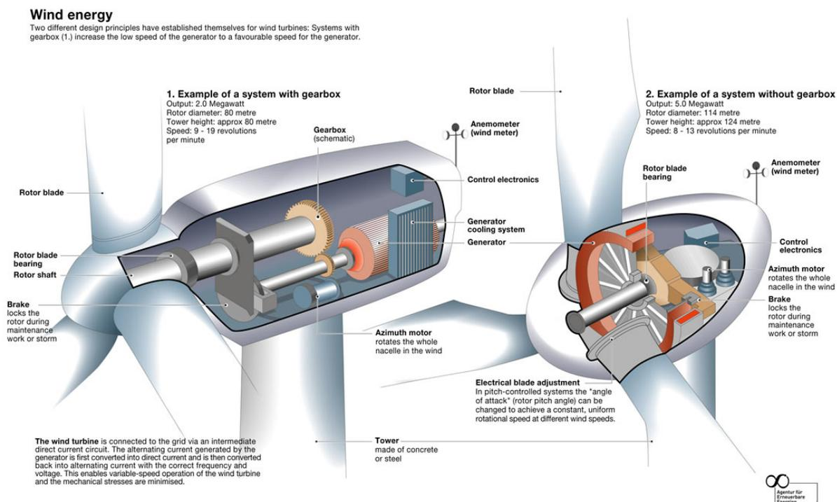
**Figure 3.44.** Comparison between a gear-box (left) and direct-drive (right) wind turbines. Source: Wikimedia. License: CC BY-SA 4.0.
