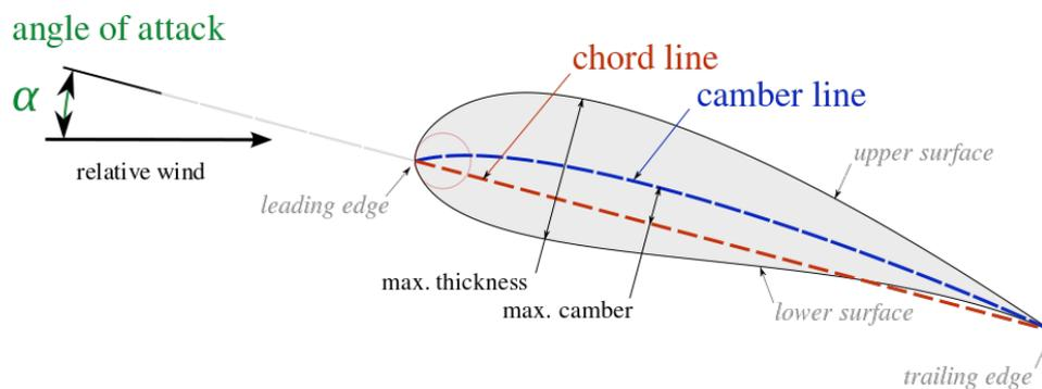
**Figure 3.21.** Plane wing profile (aerofoil). Source: Wikimedia.
