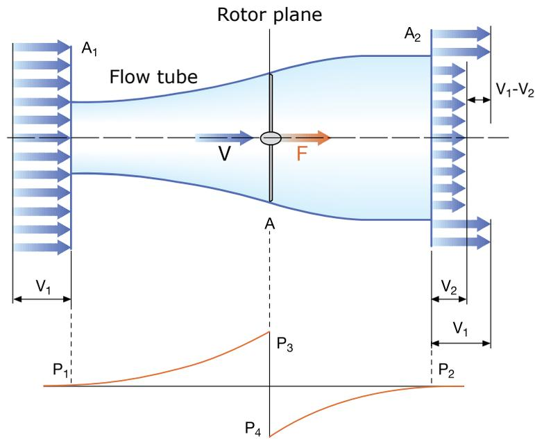
**Figure 3.17.** Variations in the speed and pressure of the air mass that goes through the wind turbine rotor. Source: Plantas eólicas/ABB Cuaderno técnico.
