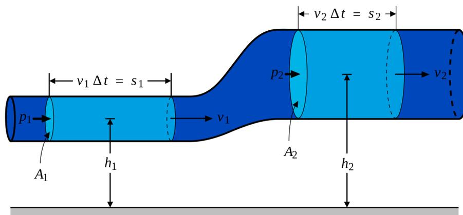
**Figure 3.19.** Schematic representation of Bernoulli's Theorem. Source: Wikimedia <http://bit.ly/2DCneFZ>
