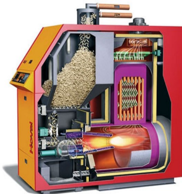
Figure 4.30. Scheme of a domestic biomass boiler. Source: http://bit.ly/2Gjping .
