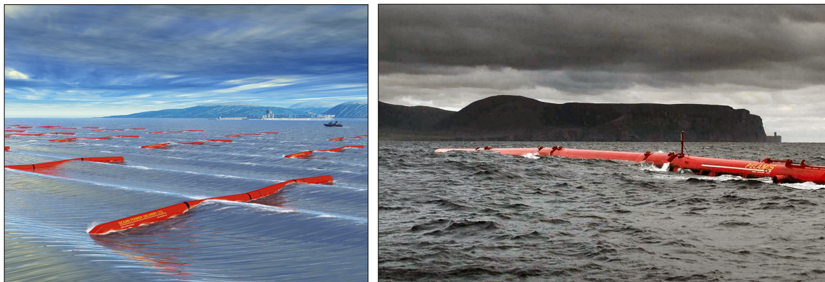
Figure 4.19. Attenuating wave energy converters: a) Pelamis wave energy plant (Source: Jumanji Solar (Flickr) http://bit.ly/2DHM9dE , b) Pelamis device tested in EMEC (European Marine Energy Test Centre) (Source: Wikimedia http://bit.ly/2rDoZjU (License: public domain)).
