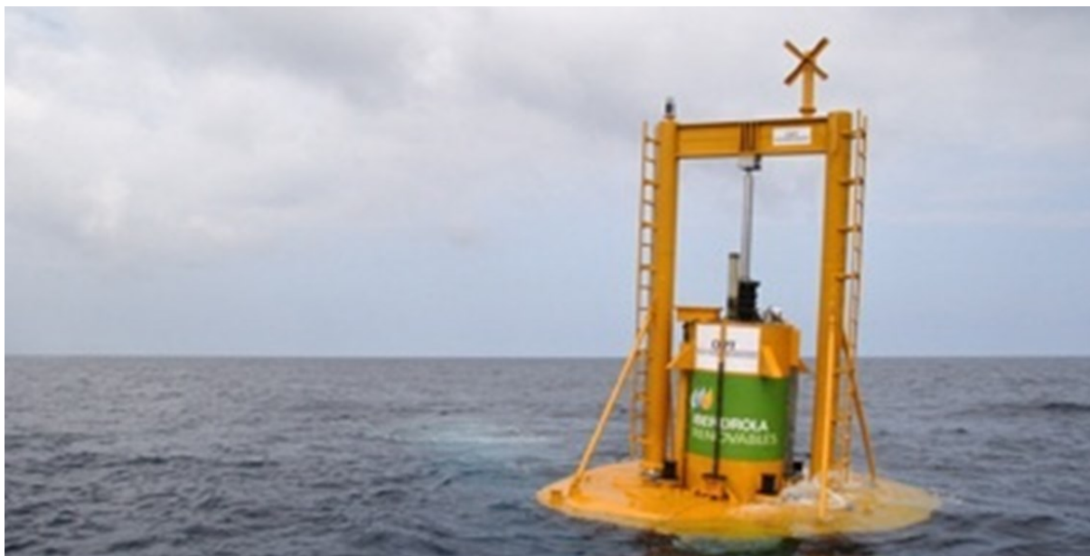
Figure 4.18. Point absorber buoy installed in Santoña (Cantabria). Source: Europapress http://bit.ly/2DBFuhC
