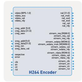
The H.264 encoders use very simple interfaces to communicate with the external host system logic and are setup by means of a simple control register set. The default values for most parameters may be pre-configured to custom specifications. Input and output data interfaces support continues streaming while also allowing the external logic to fully control the flow of data. A generic memory controller interface is used, supporting a variety of available memory controllers.
