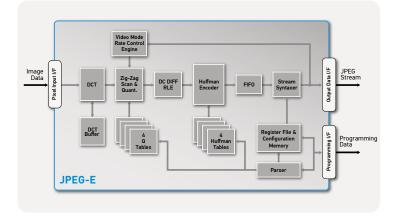
The JPEG-E and JPEG-E-X IP cores are standalone high performance JPEG encoders for still image and video compression applications.
