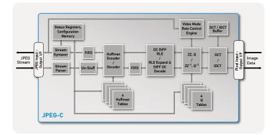
The JPEG-C core is a standalone high performance, half-duplex Baseline JPEG codec for still image and video compression applications.
