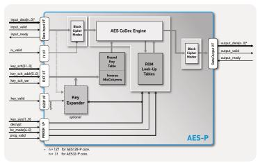
The AES-P core family implements the FIPS-197 Advanced Encryption Standard, and can be programmed to either encrypt or decrypt 128-bit blocks of data, with 128- bit, 192-bit or 256-bit cipher-key. The Block-Cipher mode of operation can also be run-time programmed to one of: ECB, CBC, CFB, OFB, CTR.
