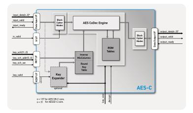
The AES-C core family implements the FIPS-197 Advanced Encryption Standard, and can be programmed to either encrypt or decrypt 128-bit blocks of data, with a 128-bit, 192-bit or 256-bit cipher-key.
