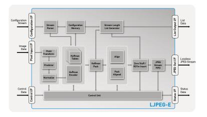
The LJPEG-E core implements the Lossless JPEG compression in a compact, high-performance, stand-alone package, ideal for applications where bit-by-bit accurate reproduction of an image is essential.
