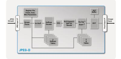
The JPEG-D and JPEG-D-X cores are standalone high performance JPEG decoders for still image and video decompression applications.
