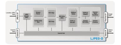
The LJPEG-D core implements a Lossless JPEG decoder in a compact, high-performance, standalone package, ideal for applications where bit-bybit accurate reproduction of an image is essential.
