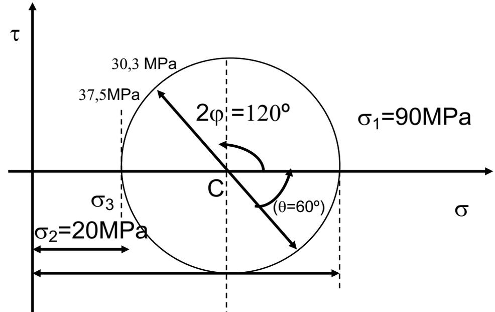
$$C = 55 \text{ MPa} \quad r = 35 \text{ MPa}$$
