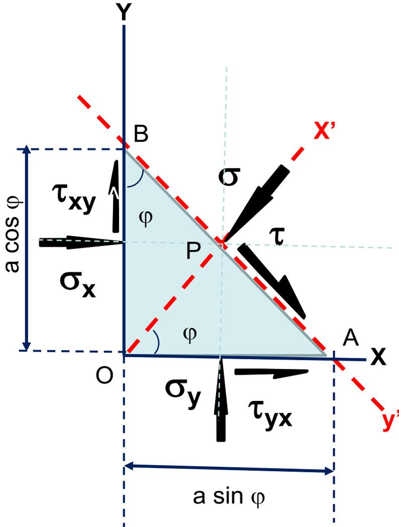
$$\sigma = \frac{\sigma_x + \sigma_y}{2} + \frac{\sigma_x - \sigma_y}{2} \cos 2\varphi + \tau_{xy} \sin 2\varphi$$
