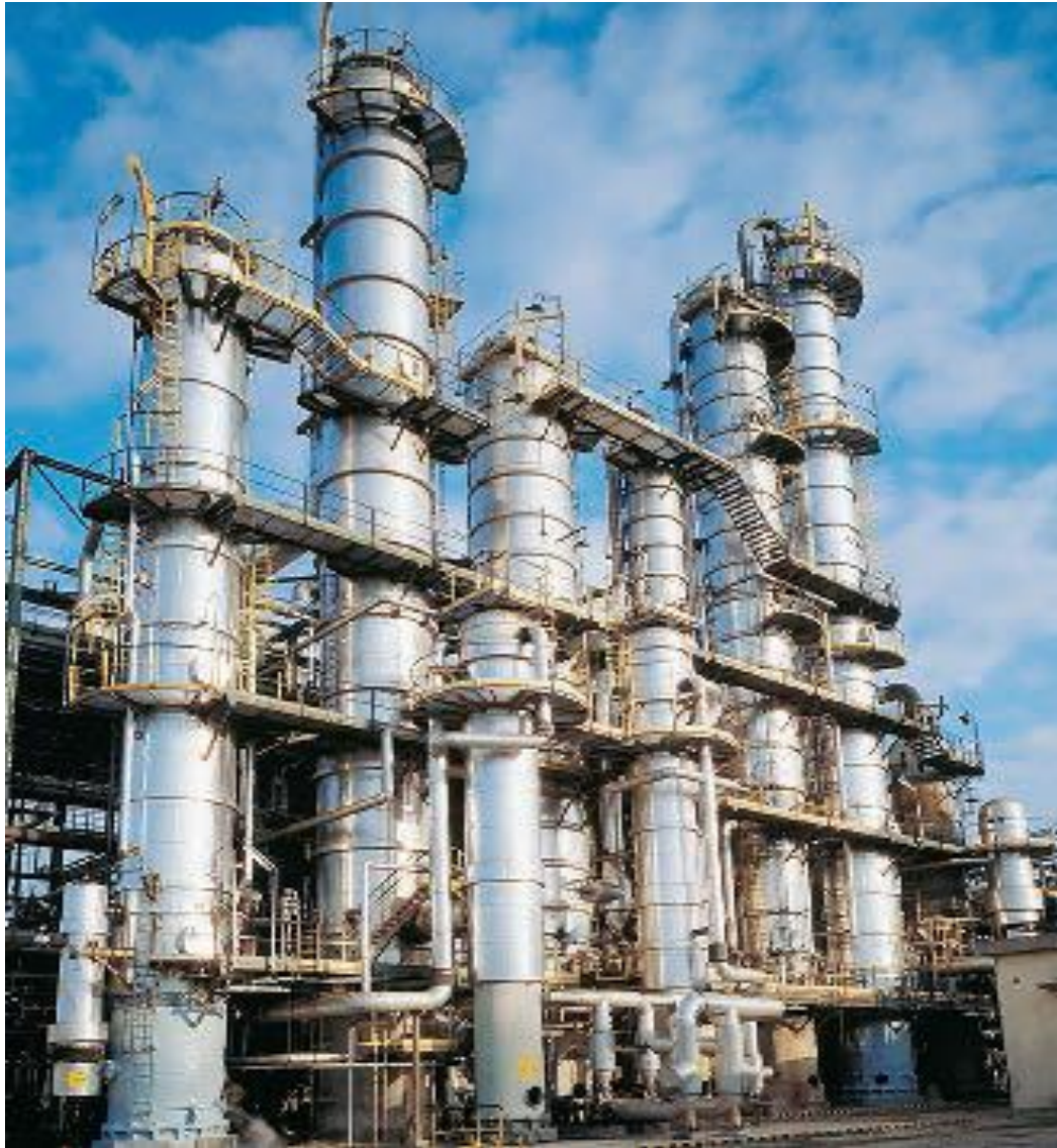
Packed bed distillation column used the in petrochemical industry. © Sulzer Chemtech Ltd., Switzerland.
