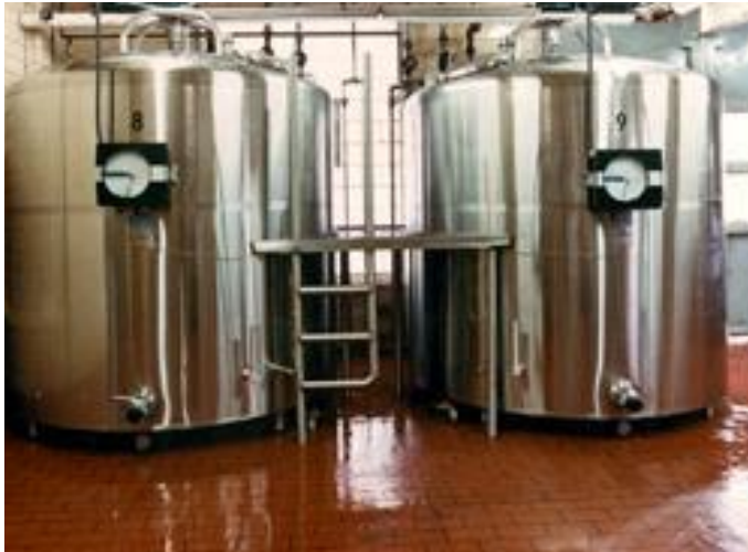
Batch reactors used in the dairy industry. © DCI Inc. St. Cloud, MN.
