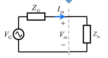
$$V_{in} = \frac{V_G Z_{in}}{Z_G + Z_{in}}$$
