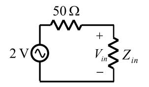
$$V_{in} = V(-l) = V_{0i} \left( e^{-j\beta(-l)} + \Gamma_L e^{j\beta(-l)} \right)$$
