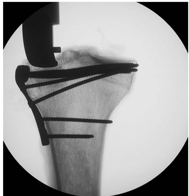
**FIGURE 6.** Specimen during destructive loading. Specimens failed through 10 mm migration of the plateau, as shown in this radiograph.
