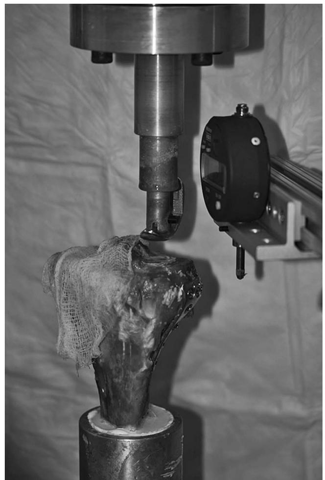
**FIGURE 1.** Biomechanical setup, including a dial indicator mounted rigidly to the test frame.
