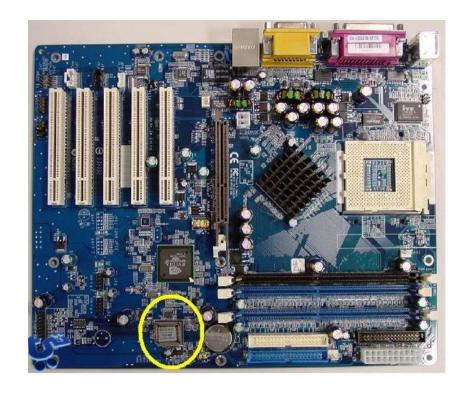
Such direction corresponds to an EPROM/Flash (motherboard) that stores the code corresponding to the Firmware (memory-mapped I/O).
